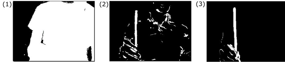
*Fig. 4:* Analysis of movement with difference-images, (1) With background as reference-image, (2) With three following images, movement of the body, (3) With three following images, only movement of the arm
