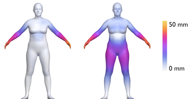
Figure 11: Comparison of our localized shape modification (left) with a global PCA approach [PSR*14] (right). Both models were used to shorten arm length by 38 mm. The vertex distance from the original to the modified mesh is color coded. Our model enables more localized shape changes, while the global PCA approach considerably changes the leg region when modifying arm length.
